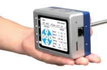
The Micro 5-Hole Probe Anemometer (WTN MPS) is a compact and lightweight device for measuring airflow pressure, velocity, and direction, with built-in advanced algorithms for 5-hole probes, and is characterised by high accuracy, stability, and performance, mainly used for flow field tests such as aircraft attitude and velocity tests, impeller mechanical flow tests, and wind tunnel tests.
